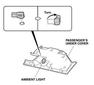
18. Reinstall the dashboard passenger's side panel.
