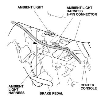
11. Plug the ambient light harness 2-pin connector into the ambient light.
