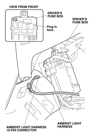
8. Secure the ambient light harness to the vehicle harness with one wire tie.
